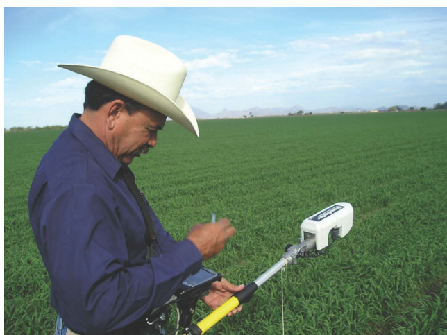
IMAGE 5.4. Infrared Sensor Technology Increases the Cost-Efficiency of Nitrogen Fertilizer Applications in the Yaqui Valley
