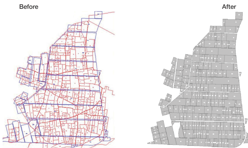
FIGURE 13.7. Parcels Before and After Land Consolidation with New Irrigation Network
